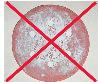
Despite a longer curing time with other products, only the surface is cured and the sanding paper becomes clogged.
